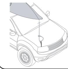
Bow and stern tie-downs are required when transporting boats. If your vehicle does not have a tie-off point or the tie-down would damage the vehicle, then Hood Anchor (Yakima part # 8007416) MUST be used. If these options do not work, please contact Yakima directly to discuss alternative solutions.
